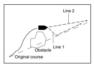
Figure 7-7 Example of when to restart navigation
